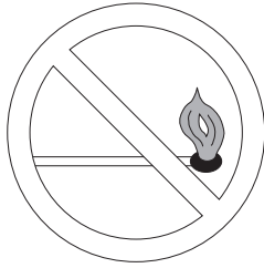
Fig. 3 - Do Not Light Burner with Match
